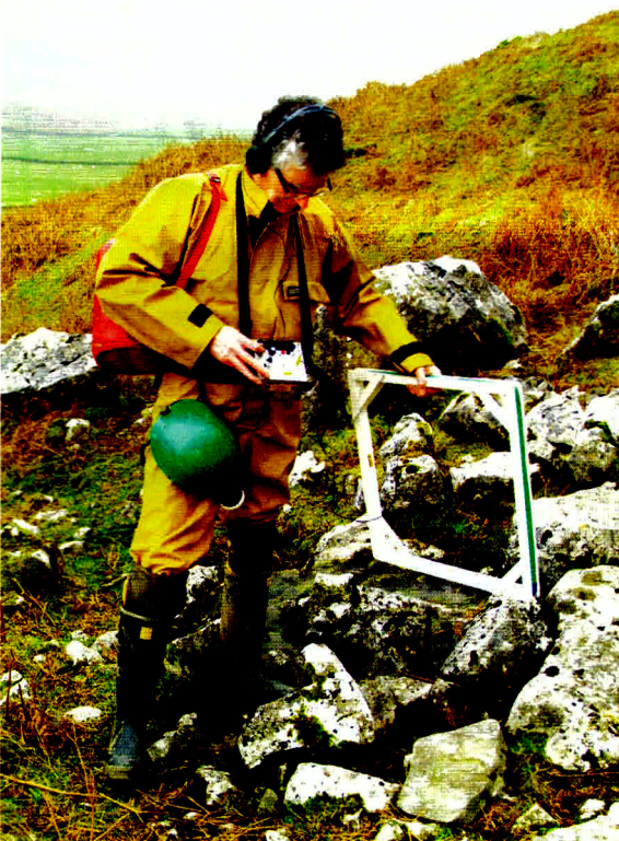
This radio location receiver is able to pinpoint an underground transmitter to provide a fixed point on the surface.
