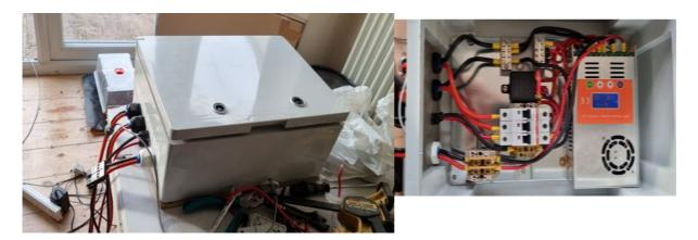
The charge controller box is new and has been calculated to naturally cool the charge controller without being open, however if the marketing department's efficiency claims are very wrong the controller may overheat when under high load. Like when first charging the battery after the winter. Please monitor it, no more than 50degC inside (This is nearly too hot to touch). If there is a thermal problem I will have to rethink the cooling...
