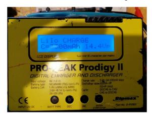
If so hold down the 'Enter, Start Stop' button for two seconds. The screen will display 'battery check' and then start charging. The screen will look something like below (but with different numbers) when charging.
