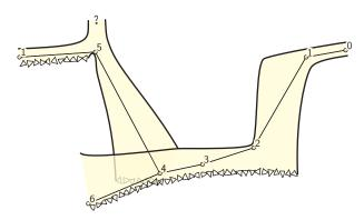
The only thing that is missing is connection line between stations 1 in these two branches. Therion does not automatically generate these lines because their shape usually depends on particilar map.
