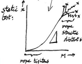
Self weight of rope is ignored throughout. OK, but 300m of wet rope is a significant weight ....
